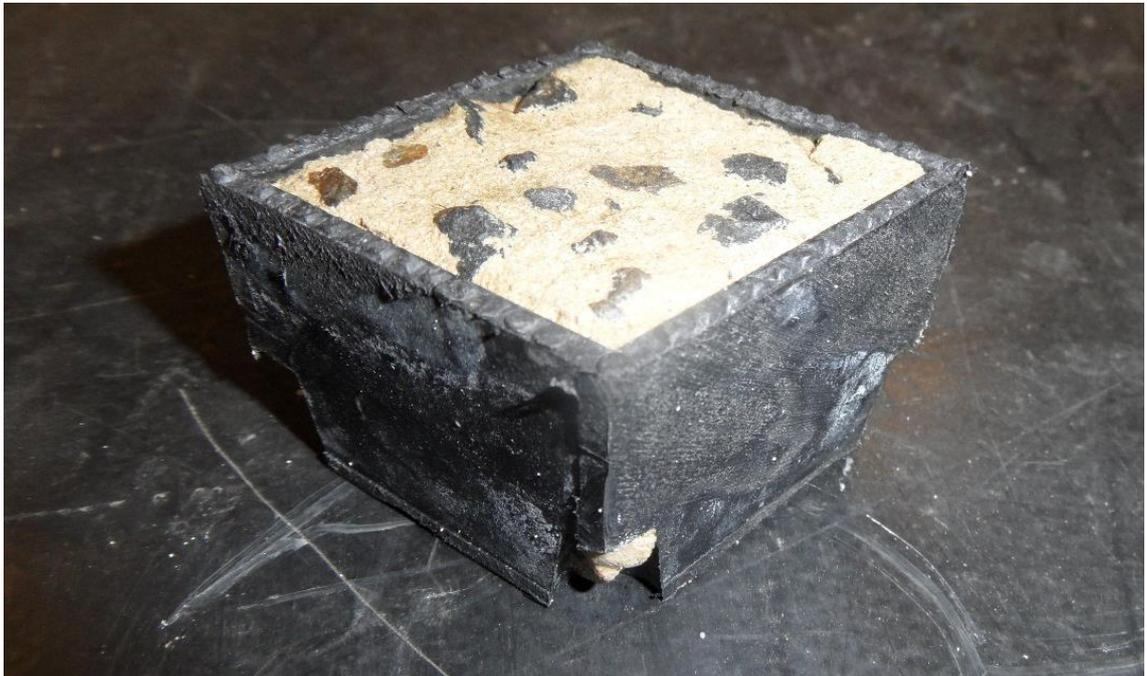
Figure 2: Testing configuration A - a single cell of the grid was extracted and the compression stress of the unit assessed.
